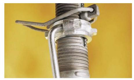
The drift pin can be released with a single hammer blow, automatically lowering the prop by 3/8 in. (9.5mm). Removal has never been faster or easier. And the integrated pin retainer means that it can never be lost or misplaced. In fact, all post shore components are interlocked so that workers don't waste valuable time sorting or searching for parts. The L-shaped handle provides easier fine adjustments of the prop.
